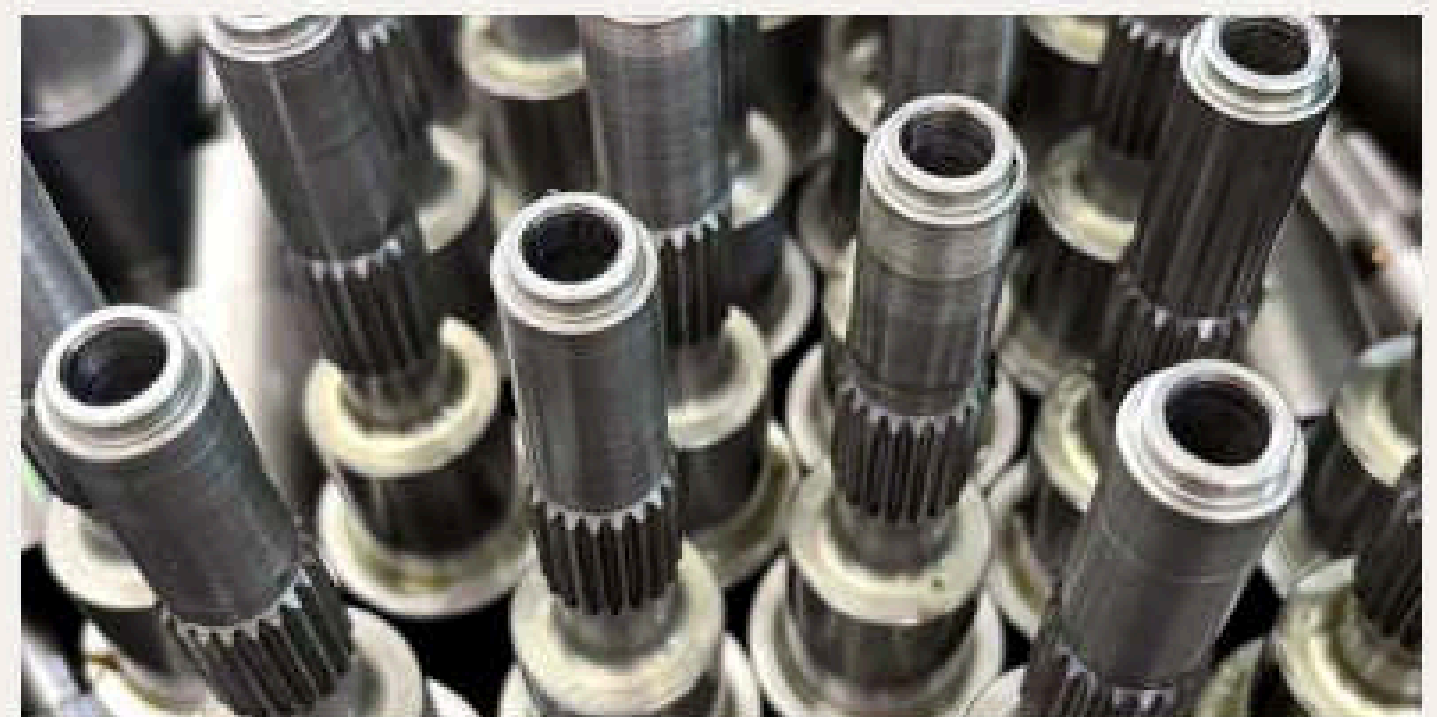
Spline and gear shafts machined complete in one setup
