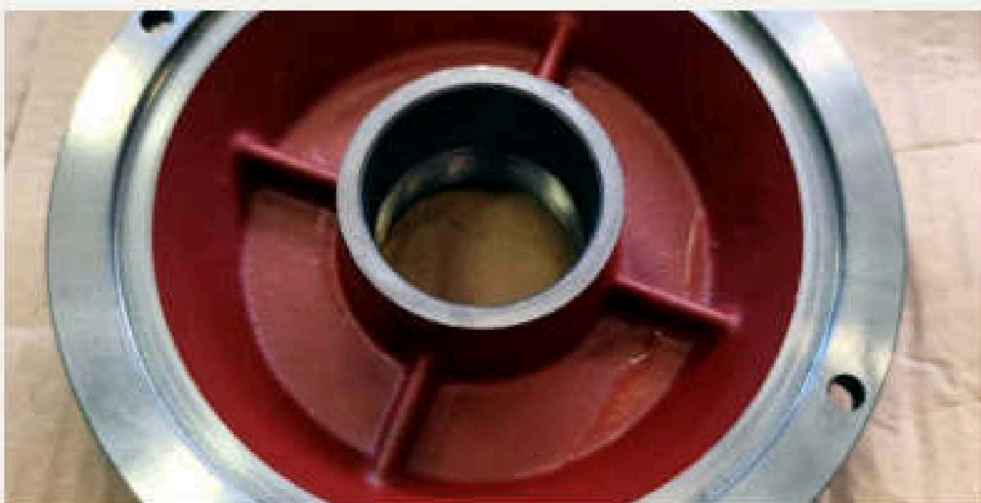
Fully machined cast bearing cap — bore, face and threads
